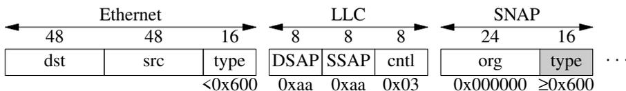
When an 802.1Q header is inserted after the Ethernet source and destination, this field is populated with the encapsulated Ethertype, not the 802.1Q Ethertype. With an Ethernet II inner frame, the result looks like this:
