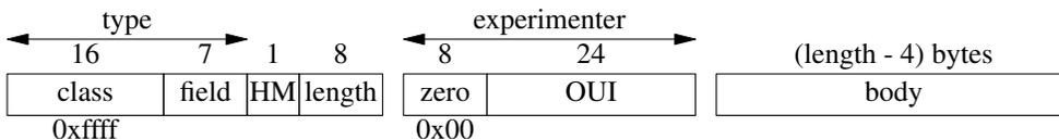
OpenFlow says that support for experimenter fields is optional. Open vSwitch 2.4 and later does support them, so that it can support the following experimenter classes:
