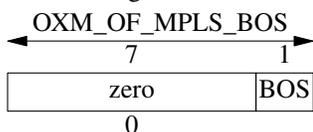
This field is useful as part of processing a series of incoming MPLS labels. A flow that includes a **pop\_mpls** action should generally match on **mpls\_bos**:
