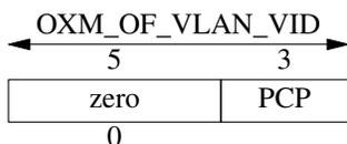
This field may only be used when **vlan\_vid** is not wildcarded and does not exact match on 0 (which only matches when there is no 802.1Q header).
