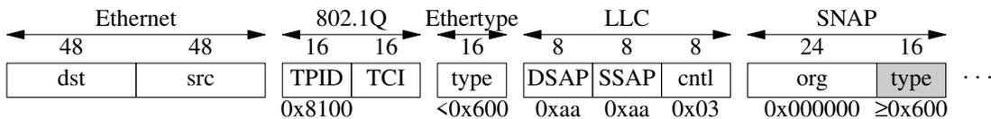
When a packet doesn't match any of the header formats described above, Open vSwitch and OpenFlow set this field to **0x5ff** (**OFP\_DL\_TYPE\_NOT\_ETH\_TYPE**).
