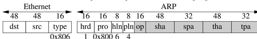
The ARP fields are also used for RARP, the Reverse Address Resolution Protocol, which shares ARP's wire format.
