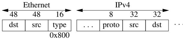
The latter is an IPv4 packet not encapsulated inside any outer frame, like this:
