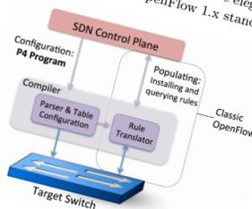
Figure 1: P4 is a language to program packet processors in a way that is independent of the hardware and software vendors.
